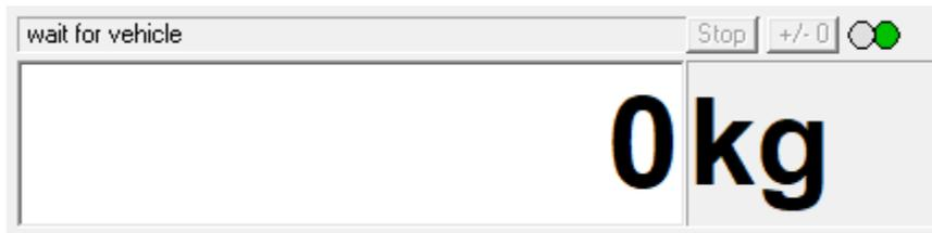
In the upper right corner of the main window, the current load of the scale is continuously displayed. In weighing mode, this value can also be seen on the external display. In weighing mode, additional information can also be output in this field and thus also on the additional display in order to give instructions to the driver. See "Information on the external display".
