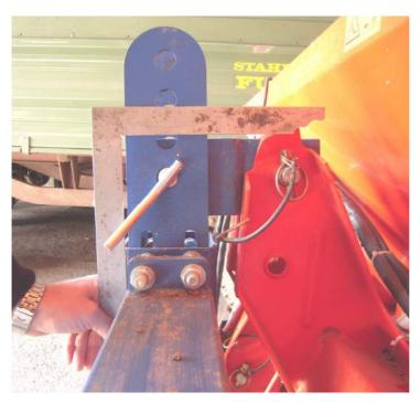
A correct setting of the mounting height is of paramount importance for your scale's accuracy.
