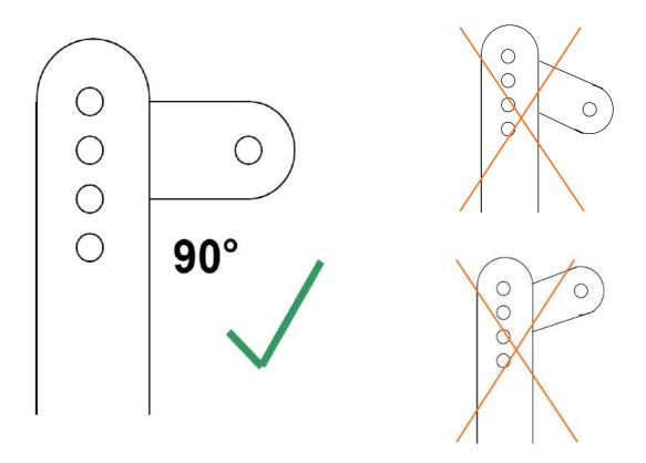
ATTENTION: The exact setting of mounting height is not only a prerequisite for accurate weighings. When the angle is not exactly right, the three-point scale and/or your implement could get damaged or deformed.
