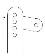
If the scale displays a higher weight in the front, you must shift the two mounting parts slightly downwards. You do not have to remove the scale. Loosen the 4 internal nuts of the mounting screws and tap the top of the sliding mounting parts with a rubber hammer. If you can't slide them any further, you have to remove the scale and insert the upper link pin in the next hole.
