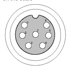
Front view cable plug on the connecting cable
