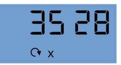
The sum of the counted revolutions is displayed, the symbol with the rotary arrow and the x light up.
