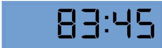
If the colon is visible as separator, it is hours and minutes.
